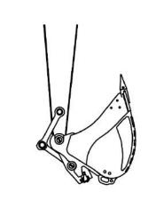
Once the front bosses are in the front wedge lock hook, start to curl the coupler and attachment in. You may have to lift the boom a little to allow the coupler and attachment to curl in. Curl the coupler and attachment all the way in, so that the weight of the attachment is on the coupler, and the rear coupler boss is now contacting the wedge lock hooks. (See picture to the left)
