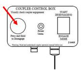
NOTE: The control box will lock out if you wait longer than 5 seconds to hit the button. If that happens, flip the rocker switch back to "ENGAGE MODE". Within 5 seconds of flipping the rocker switch, press and hold the disengage button for at least 2 seconds (see picture to the left). **The buzzer will start to beep once every second, and the button will start flashing.** Hold the bucket curl cylinder over relief for at least 5 seconds until you see the coupler fully unlock.
