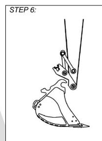
Once the rear of the coupler is free from the attachment, continue to curl the coupler all the way out. Now, pull the front bosses of the coupler out of the front wedge lock hooks. Sometimes this is easiest to do by curling the stick in and dropping the boom. (See picture to the left)
