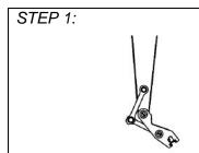
To unlock the coupler to get it ready to engage an attachment, the first thing that will need to be done is curl the coupler all the way in, as shown in the picture to the left.
