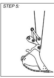
Lower the attachment close to the ground and curl the coupler out. At this point, the rear of the coupler should come free from the attachment. (See picture to the left)
