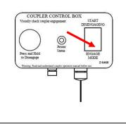
Once the coupler and attachment are curled in, and the rear boss is now hitting the wedge lock hooks, flip the rocker switch to "ENGAGE MODE". (See picture to the left) **Once the rocker switch is flipped**, **the buzzer will shut off and the control box will revert to idle mode**. Continue to hold the bucket curl over relief for at least 5 seconds until the coupler locks.
