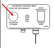
NOTE: The control box will lock out if you wait longer than 5 seconds to hit the button. If that happens, flip the rocker switch back to "ENGAGE MODE". Within 5 seconds of flipping the rocker switch, press and hold the disengage button for at least 2 seconds (see picture to the left). **The buzzer will start to beep once every second, and the button will start flashing.** Hold the bucket curl cylinder over relief for at least 5 seconds until you see the coupler fully unlock.
