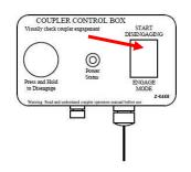
Once the coupler is curled all the way in, flip the rocker switch to "START DISENGAGING", as shown in the picture to the left. At this time, the buzzer will start sounding constantly, and the button will light up.
