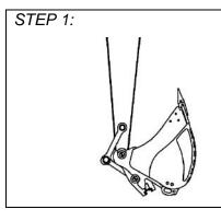
To unlock the coupler to get it ready to drop off the attachment, the first thing that will need to be done is curl the coupler and attachment all the way in, as shown in the picture to the left.
