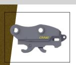
The Craig TrueGrip pin grabber has a simple and reliable design. It features 2 independent locks and has visual safety indicators that allow the operator to ensure both the front locking knuckle and rear latch are engaged. Works with most OEM Coupler Kits (confirm with Craig) or can be supplied with a Craig hydraulic kit.
