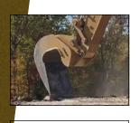
The rock slab bucket expertly gets under layers of rock to break and remove chunks and slabs of rock. The half arrow tip and smooth edge makes it easy to slip between layers of rock to pry and lift slabs.
