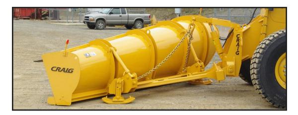
One of the most common grader attachments is a one way plow. The 1073-10 plow is shown here with a standard chain lift on a Deere G series grader. Note the chains are slack at ground height and the harness is bolted on using the lower holes on the Deere G series head block.
