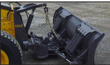
The 850 series dozer blades attach onto the 100 plow harness in much the same way a DPF reversible plow does. Shown here is a Cat 140M grader. Dozer blades are meant to work on a hydraulic circuit with hydraulic float which is why the down pressure arms do not have mechanical float slots like the slotted reversible plow down pressure arms.
