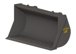
Available in 56" and 72" widths, the Craig Mulch Bucket provides an accurate struck capacity of 1.00 cubic yard. (1.19 cubic yards heaped). The deep narrow design allows for accurate loading of quarter ton or half ton pickups in the commercial sale of mulch.
