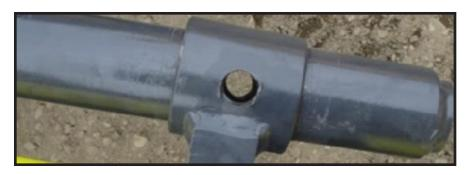
When the collar on the lift group and the adjustable brace are lined up the locking pin can be inserted.
