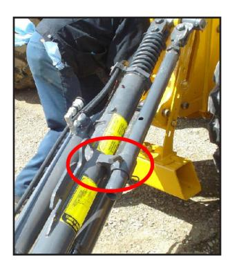
Shown above is the pin in its locked position. The rear lift group can now be raised rigidly with the wing moldboard detached.
