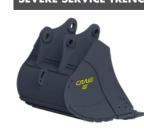
Craig Severe Service Buckets are specifically designed to meet your toughest applications. Superior Brinell 400 quenched and tempered steel is used in the main-sheet, end-plates, horizontal wear bars and base edge.
