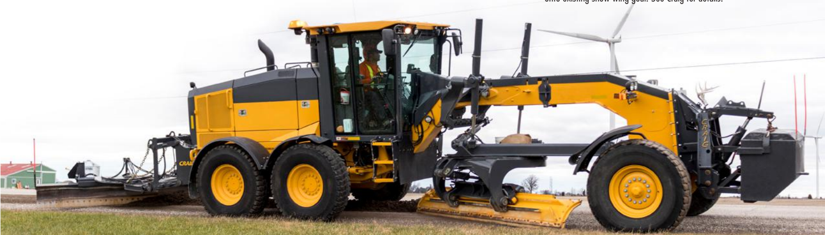
A grader equipped with a Series II Windrow Eliminator and Craig plow harness.
