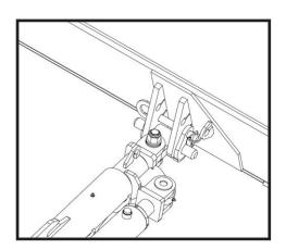
3. Before raising the wing ensure that the pin holding the adjustable brace onto the push pole is pulled as shown below. Failing to do so can cause the adjustable brace to bend or break. This brace is only intended to provide stability to the push pole when detached from the wing moldboard.
