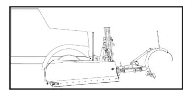
2. Unpin the wing moldboard from the push pole. The push pole will have a tendency to want to swing ahead after being unpinned, so it is important to hang onto it. After unpinning the push pole, be sure to put the pin through the adjustable brace to keep the push pole from swinging ahead into the cab of the truck when raised.
